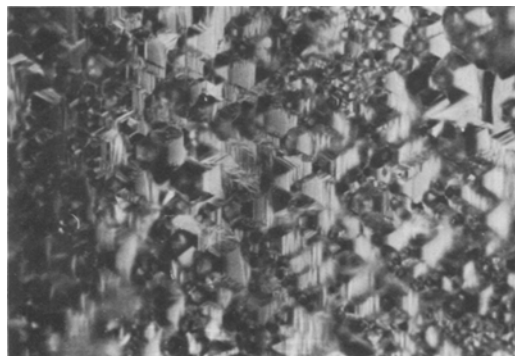
Figure 2 Chemical-etching figures on the outer face (Cd face) of a CdS layer. Etching solution: 37% HCl, × 300.
